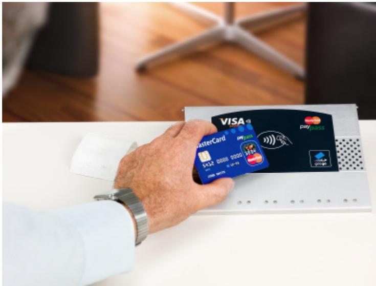
Contactless EMV-enabled credit cards and NFC-capable smartphones can communicate and exchange data with a payment terminal when the two are in close proximity.
